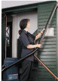
Use tank for high and detail vacuuming
